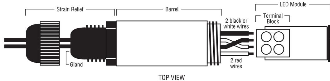
6. Bring both the incoming power wire, and the outgoing power wire, into the LED Disc Light strain relief by pushing each through the respective hole in strain relief rubber gland. If you encounter difficulty inserting wire into the gland, apply a small amount of Vaseline on the outside of the wire. Once through the strain relief gland separate the incoming and outgoing power wires into two sets of black or white and two sets of red wires. See diagram above.
