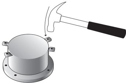
5. Select a mounting location for the Xenon Wall Light. Fixture should be within reach of 110V power, located approximately 9 inches above the surface to be lit, and situated at the best location along the mounting surface for the illumination task.
