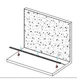
Insert the LED Wall Washer in the mounting clips.
