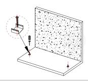
Install mounting clips with the screws provided.
