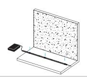
Power the LED Wall Washer with the 24V DC driver.
