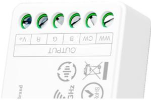
2. Connect the input side of controller to appropriate size of 24V power supply. Use EITHER the V+, V- terminals OR the barrel socket, but not both. See our Tape Selection guide for more driver information. (website)
