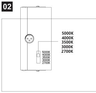
3. Set the dip switch to the desired color temperature level.
